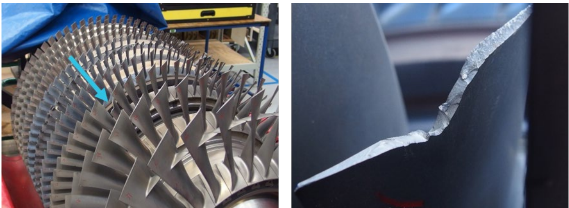
Figure 5: Stage 5 blade fatigue failure
