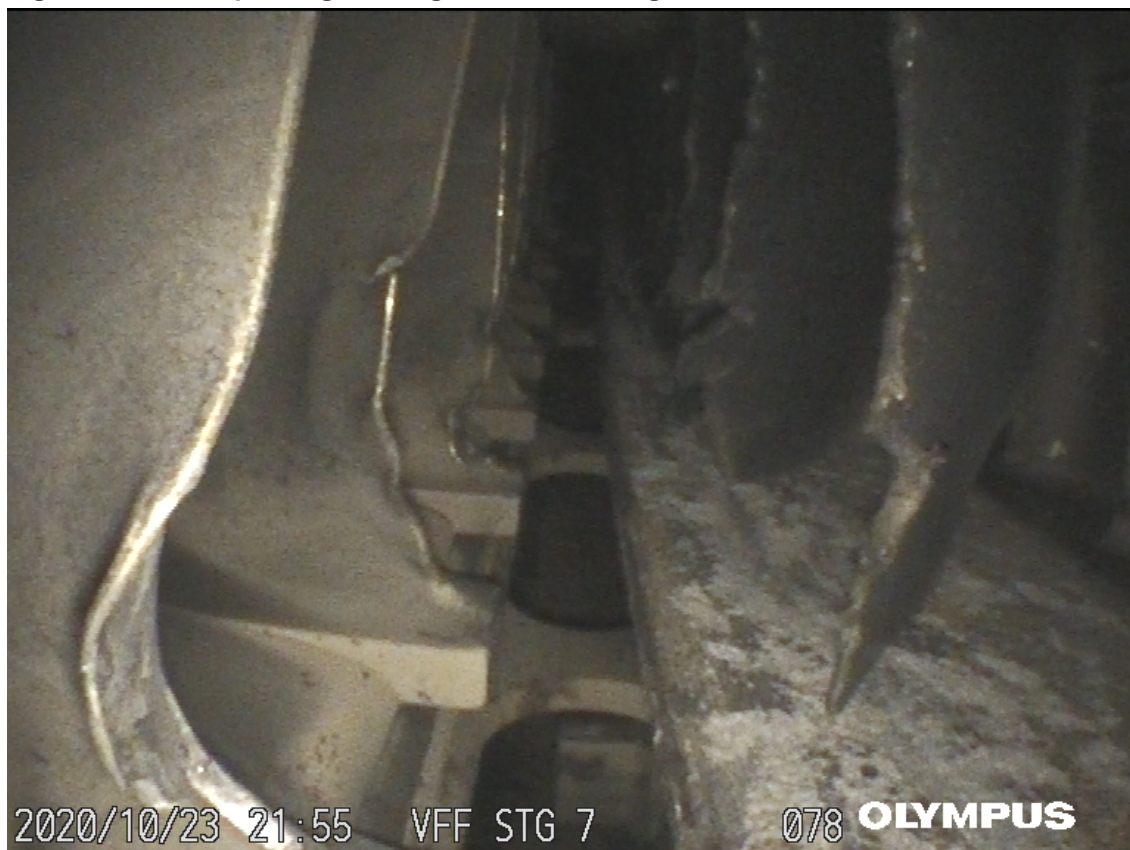
Figure 3: Borescope image of stage 7 HPC and stage 8 stator vanes
